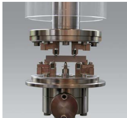
Fig. 1: 4-point flexure specimen gripping unit for dental ceramics
