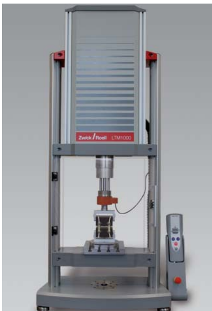
Fig. 1: LTM1000 with spinal implant
