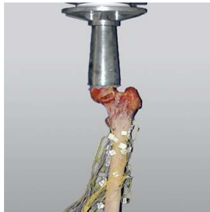
Fig. 1: Femur with strain gages applied
