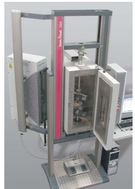
Fig. 3: Temperature chamber integrated into materials testing machine
