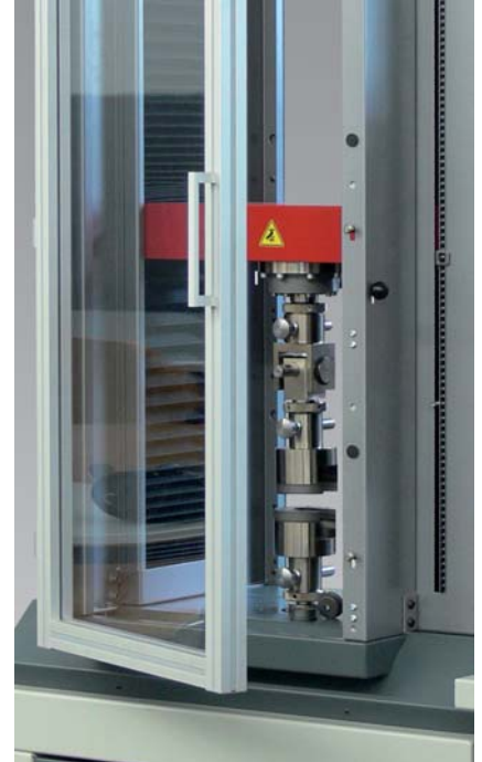
Fig 2: ProLine Z050TN with CE conforming protective screen
