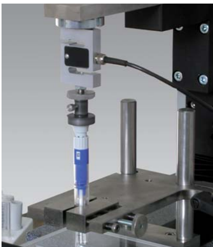
Fig. 1: Discharging device for testing insulin pens
