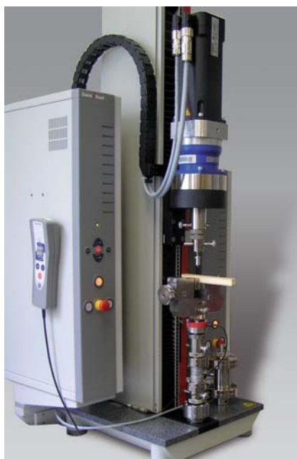
Fig. 3: zwicki-Line with torsion drive
