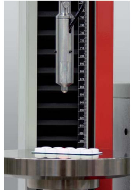
Fig. 2: Testing device with laser positioning for push-out test
