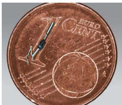
Fig. 1: Titanium stapes prosthesis (Heinz Kurz GmbH Medical Technology)
