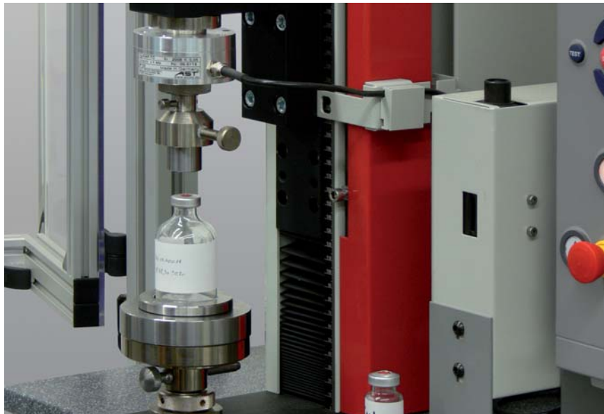
Fig. 1: zwicki-Line materials testing machine with residual seal force testing device
