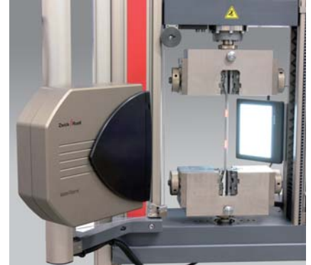
Fig 3: laserXtens with round specimen
