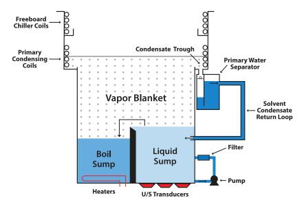
and in-line cleaning processes. The ideal vapor degreaser will be equipped with high freeboard and a secondary set of low temperature condenser coils, called Freeboard Chiller Coils, to greatly reduce diffusional vapor losses.
